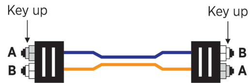
Diagram 1: A to B crossover patch cord
